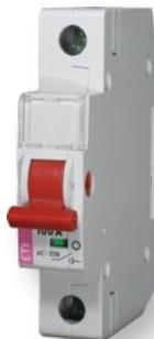
Build-in switch is used as a main switch in distribution boxes in houses or as a switch for individual electric circuits. With a build-in switch we can completely replace the cam switch. Build-in switch can be sealed either in ON or OFF position.
