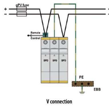
Note: If distance between string and inverter is less than 10 m, then you need only one ETITEC.
