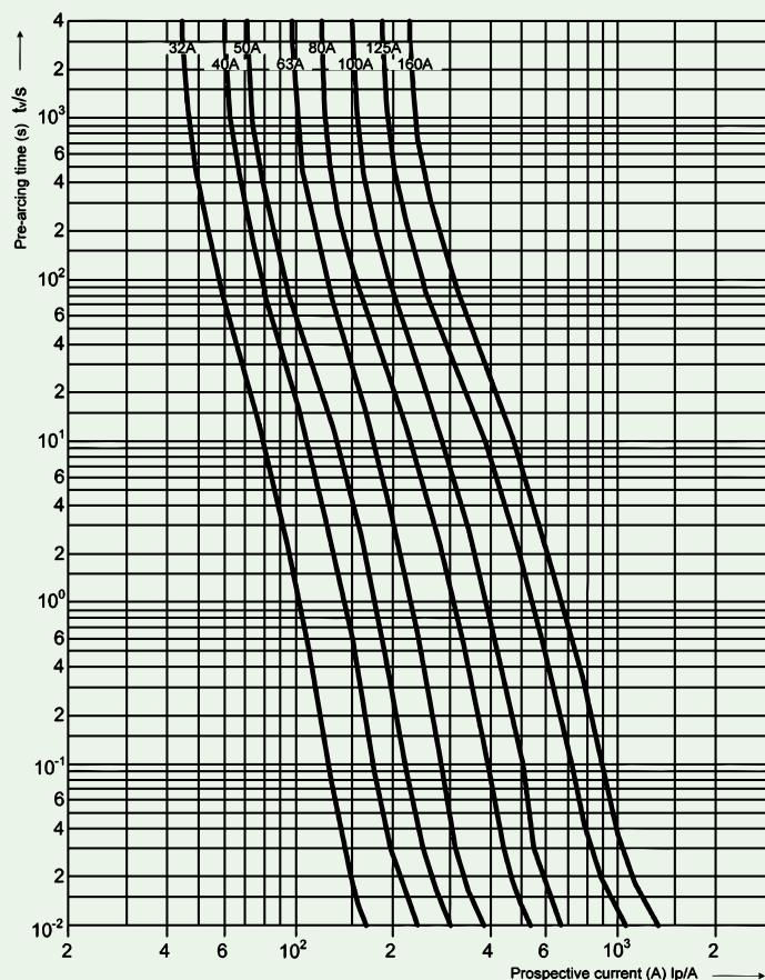
gPV, PV(gR) 750V, 1000V t-l characteristics
