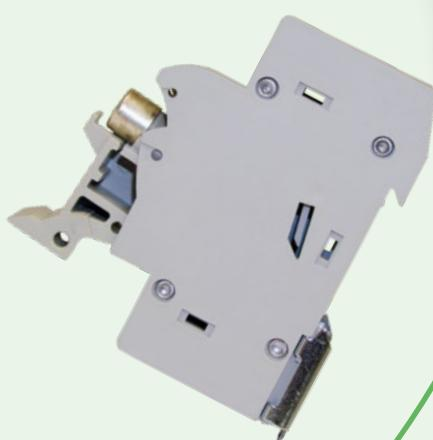
→ All plastic parts are made of material resistant to extremely high temperatures. Fuse carrier assures that a fuse link is not in touch with a housing
