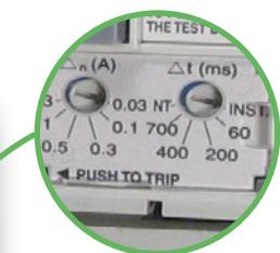
Adjustable residual current tripping thresholds between 30mA and 3A. Adjustable time delay for residual current protection between 60ms and 700ms including INST (instantaneous) and NT (No Trip).
