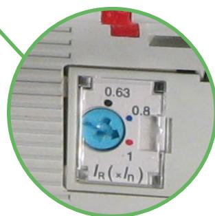
Adjustable overload protection  $I_R$  can be set between 63% and 100% of  $I_n$
